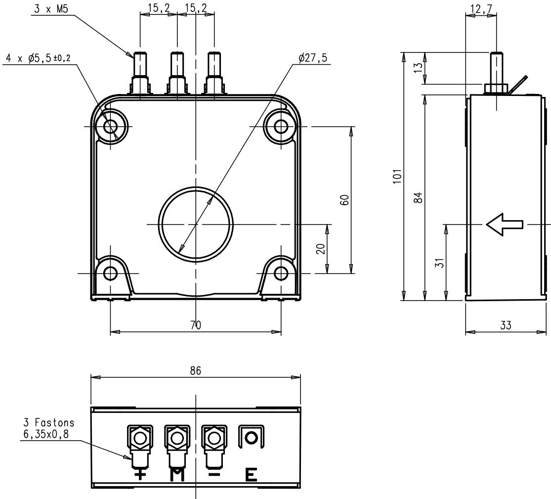
**Maximum M5 tightening torque: 2 N.m**
